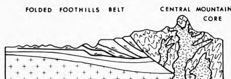
Fig. 1. A schematic transverse profile of a typical mountain range with a folded and low-angle thrust-faulted foothills belt on the left. The central mountain core is composed of intensely folded and metamorphosed rocks which have been intruded by granite batholiths.
