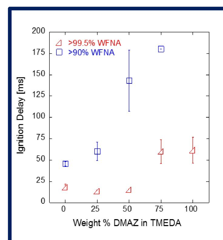
The graph compares ignition delays from droplet testing of >99.5% WFNA and >90% WFNA with a mixture of TMEDA and DMAZ fuel. Identical testing will be done on the distilled WFNA to verify it reacts similarly to the previously-purchased oxidizer as well as hotfire experiments, seen using TMEDA/WFNA > 99%.
