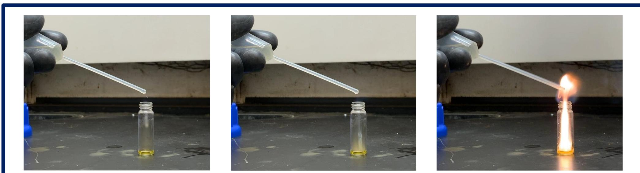
TMEDA is dropped into a pool of the distilled WFNA as a preliminary drop test to determine ignition capability. The images above are three consecutive frames, where it can be seen after impact, a luminous flame was observed. Average ignition delay time, or time from droplet impact until first light, was measured as < 33 ms.
