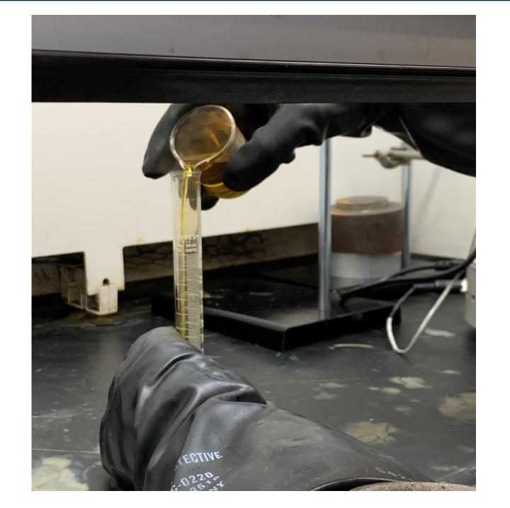
To calculate density, the mass of the WFNA had to be measured. This was done under a fume hood while protection personal wearing equipment including butyl gloves, eye protection, and a lab coat.
