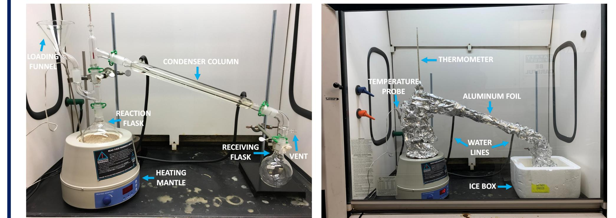
Sulfuric acid and sodium nitrate were loaded into the reaction flask. The funnel was replaced with a stopper, the heating mantle was turned on, and the setup was covered in aluminum foil since nitric acid degrades when exposed to light. The reaction produced nitric acid vapors which condensed into liquid and collected in the receiving flask. The temperature was maintained around 32 degrees Celsius for approximately 2 hours.
