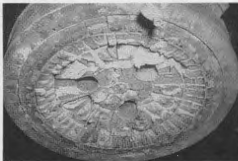
Silica Brick Roof Failure in an Electric Arc Furnace
