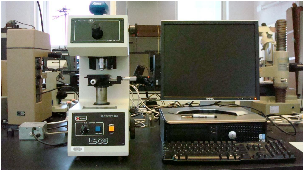
Figure 9: The Leco MHT Series 2000 Vickers Hardness Tester used to measure hardness values associated with various microstructures within the Cape York Meteorite
