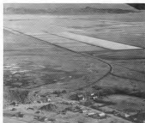
Fig. 4. Evaporation ponds of the Foote Mineral Company in Clayton Valley, Nev. These cover about 1,500 acres. Lithium-bearing brine is pumped from wells located between the ponds and the far ridge. Part of the historic mining settlement of Silver Peak is in foreground.
