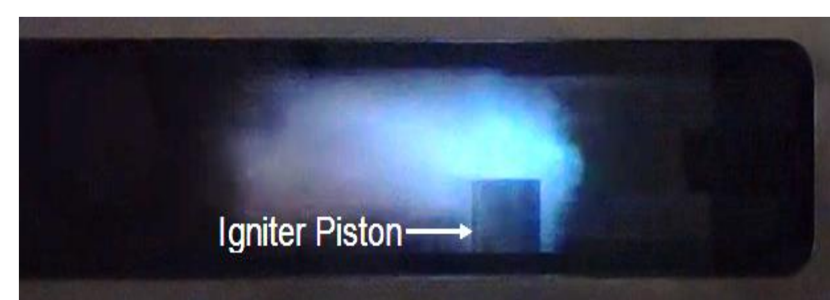
Ignition – using retractable spark plug
