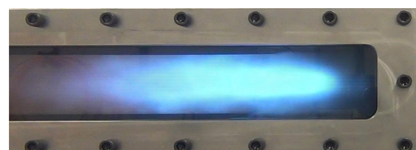
Detached Flame – pulsing flame; standoff distance from injector
