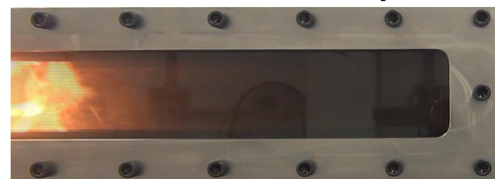
Blowoff Flame – large oscillations; least efficient; not burning all of fuel
