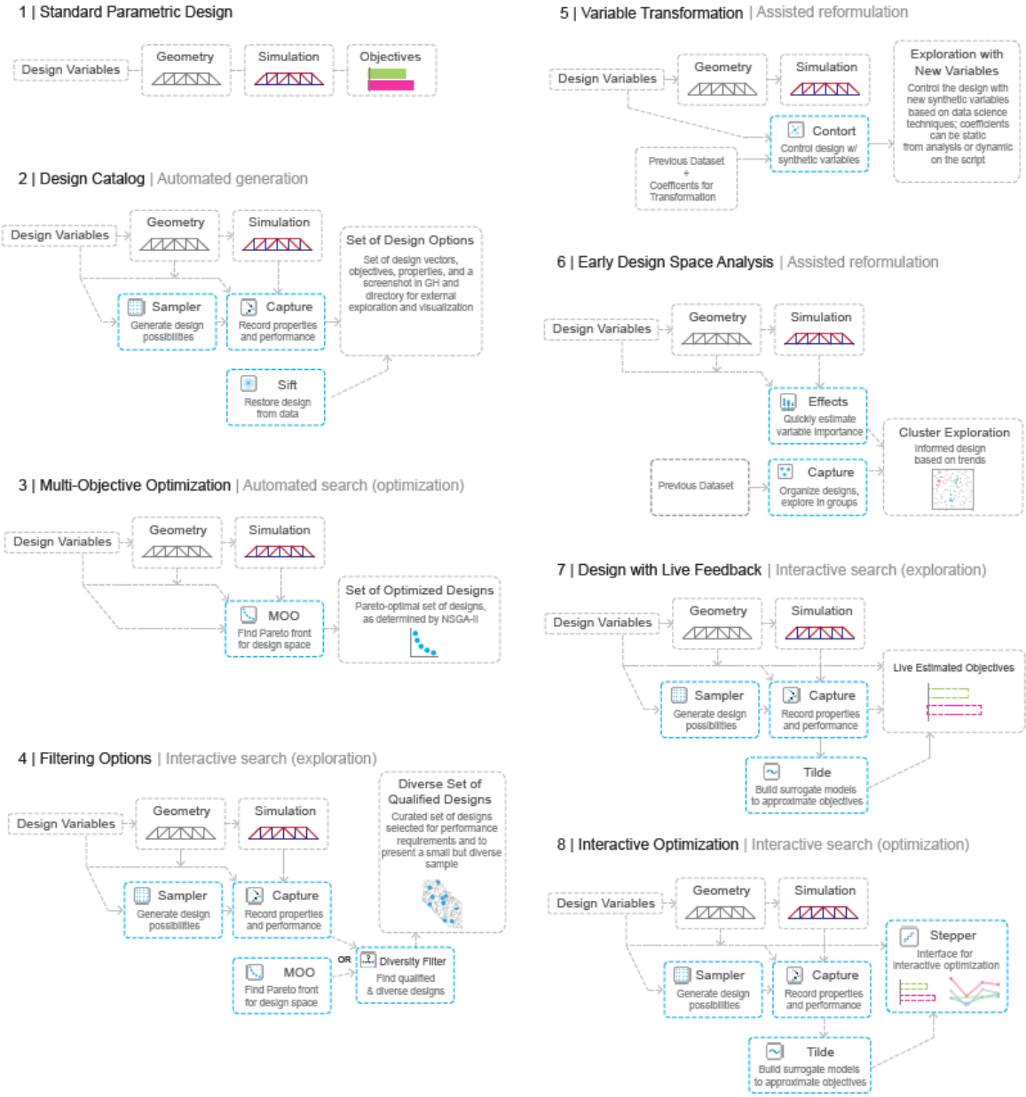
Figure 2: Different workflows enabled by the various data-driven components in DSE. Each blue box (denoted by a component logo) refers to a specific component.
