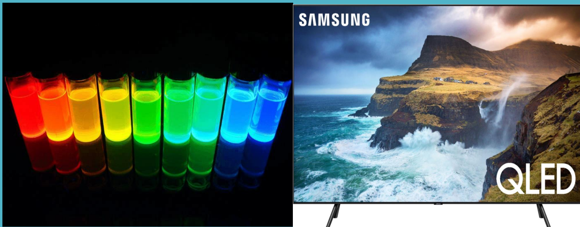
Fig 1: color emission of quantum dots and its application in television
