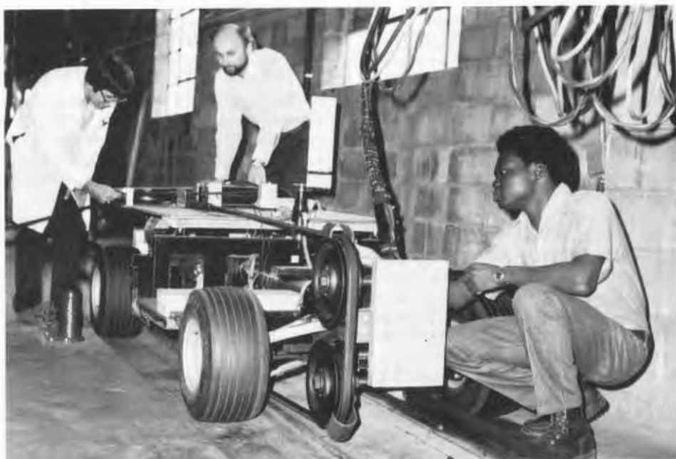
A major research area in mining engineering at Penn State in which graduate students may become involved is mine electrical systems and components. In the mine electrical research laboratory, the cart-like apparatus shown here is run back and forth to put wear and tear on the electrical cable that is wound around the vertically mounted wheels in the foreground and the horizontally mounted wheel on the rear of the cart. The object is to test the durability of splices made in the cable which is the type used to supply power to underground mining machines. Working with the cart are, left to right, George Luxbacher and Thomas Rusnak, research assistants, and Abel Folarin, a graduate student.
