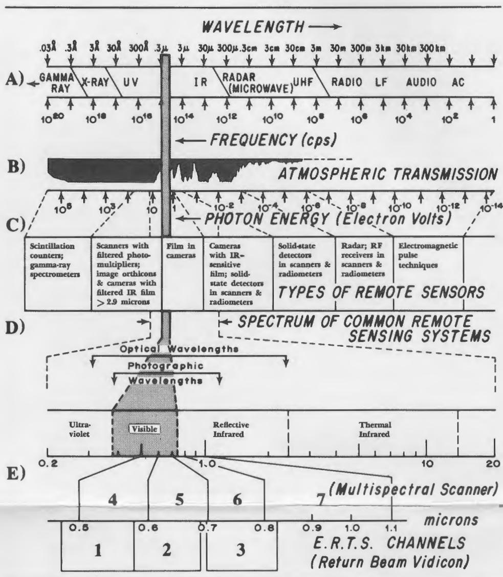
Figure 3. Range of electromagnetic radiation with appropriate detectors and the region of the spectrum pertinent to satellite and airborne sensors. (Compiled from various sources.<sup>1,2</sup>)
