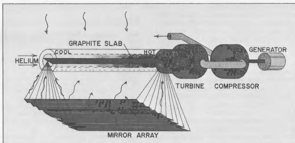
Dr. Howard Palmer's scheme for harnessing solar energy is shown in this artist's sketch. The sun's rays, striking an array of mirrors, would be reflected to pass through a glass pipe (through a slit in its insulation), and strike and be absorbed by a thin slab of graphite. Helium gas flowing around the graphite would be heated to drive a turbine coupled to a generator.
