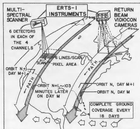
Figure 4. This sketch illustrates the principles of the camera (RBV) and multispectral scanner (MSS) systems on ERTS-1 and the ground coverage pattern. The orbit overlap is greater near the poles than over the equator.
