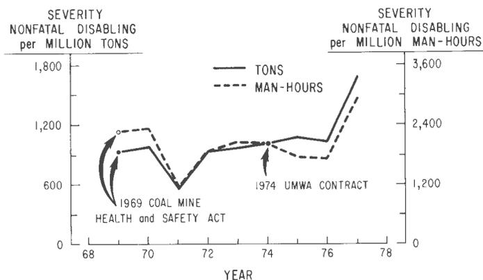
Figure 4. The severity of nonfatal disabling injuries in bituminous coal mining per million tons mined and per million man-hours worked.
