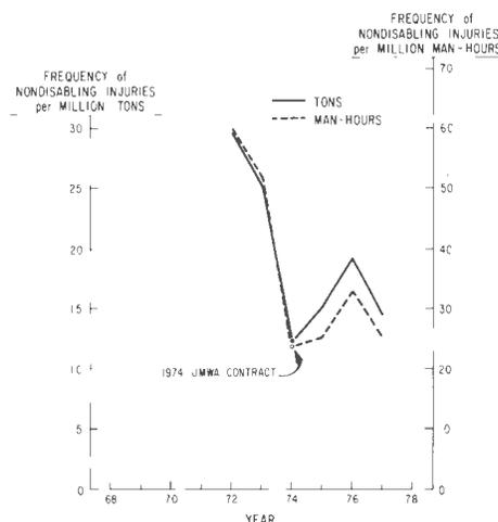
Figure 5. The frequency of nonfatal disabling injuries suffered in bituminous coal mining per million tons mined and per million man-hours worked.
