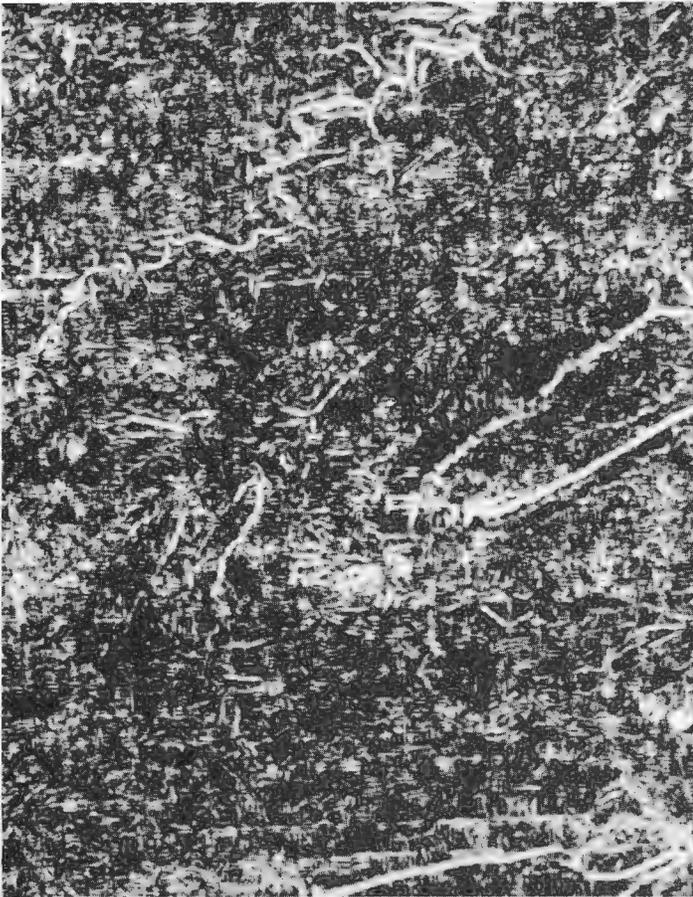
Figure 4. Gray scale map of edges showing rapid breaks in slope as white. The incomplete State College bypass can be traced as a set of edges.
