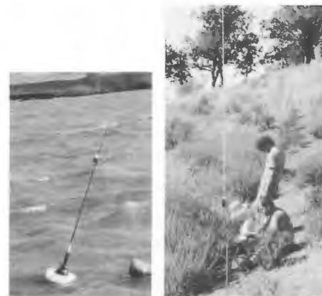
*A floating seismic transmitter (left) and (right), a seismometer site in the Bay Area.*
